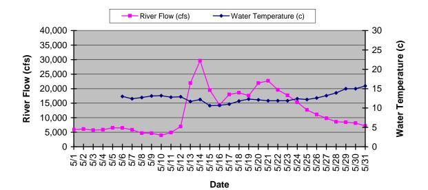
Figure 21. Water temperatures and river flows recorded at the Brunswick fishway in May 2006.
