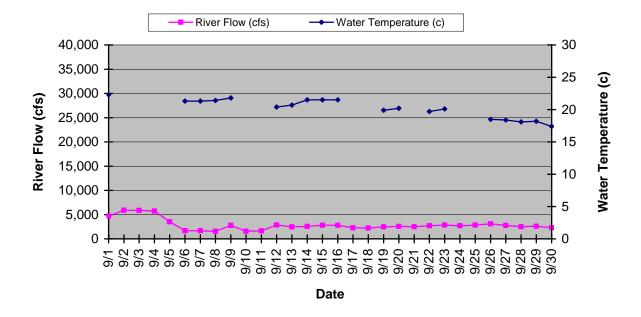
Figure 19. Water temperatures and river flows recorded at the Brunswick fishway in September 2005.
