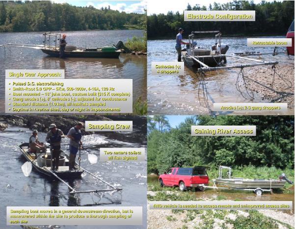
Figure I-3. Electrofishing boat and towing vehicle specifications and configuration used in the Maine rivers fish assemblage assessment, 2002 and 2003.
