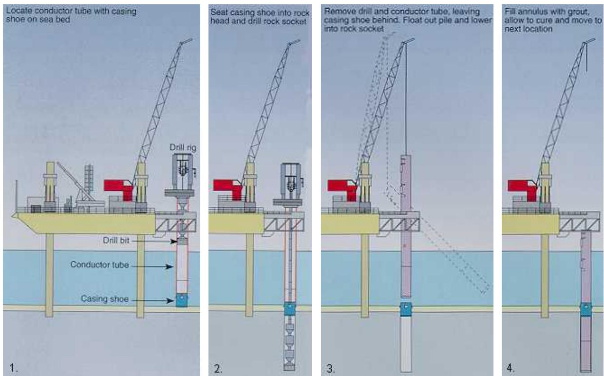
Figure 2.1-1. Monopile foundation installation sequence.
