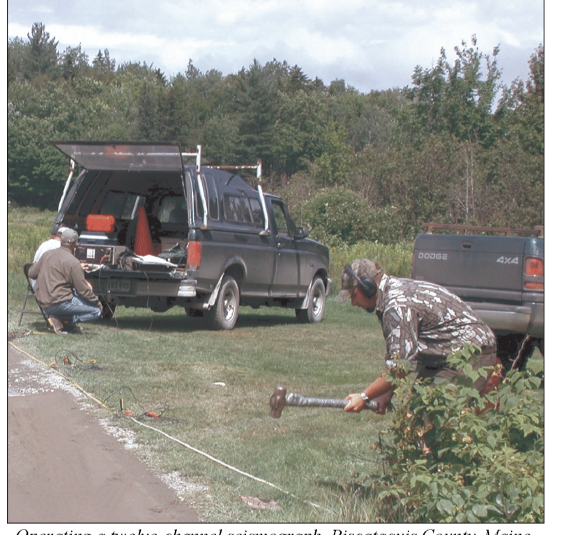
Operating a 12-channel seismicograph, Piscataquis County, Maine.
