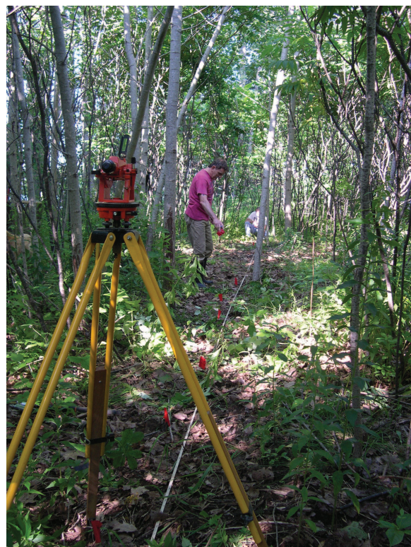
Figure 2. Laying out grid with tape and transit.
