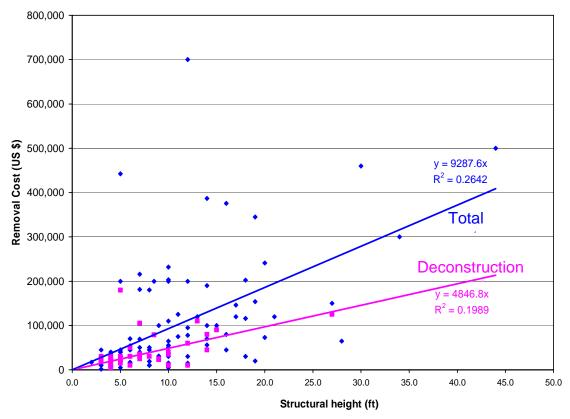
Figure 2.4 Removal cost of low head dams or small dams of different structural heights.
