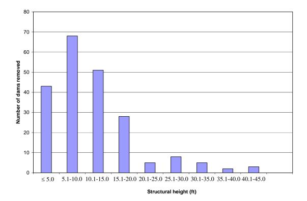
Figure 2.3 Number of removed low head dams or small dams of different structural heights.
