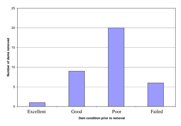
Figure 2.6 Number of removed low head dams or small dams at different conditions prior to removal.
