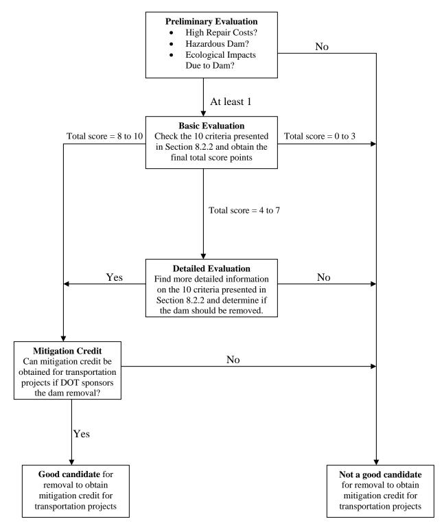
Figure 8.1. Flow chart for determining a dam candidate for removal to obtain mitigation credit for transportation projects.
