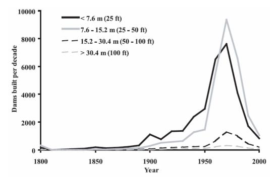
Figure 1.1 Number of dams constructed over the past 200 years by decade and by National Inventory of Dams height class (FEMA, 1999). The most active period of dam building occurred between 1950 and 1970, and has been called "the golden age of dam building."
