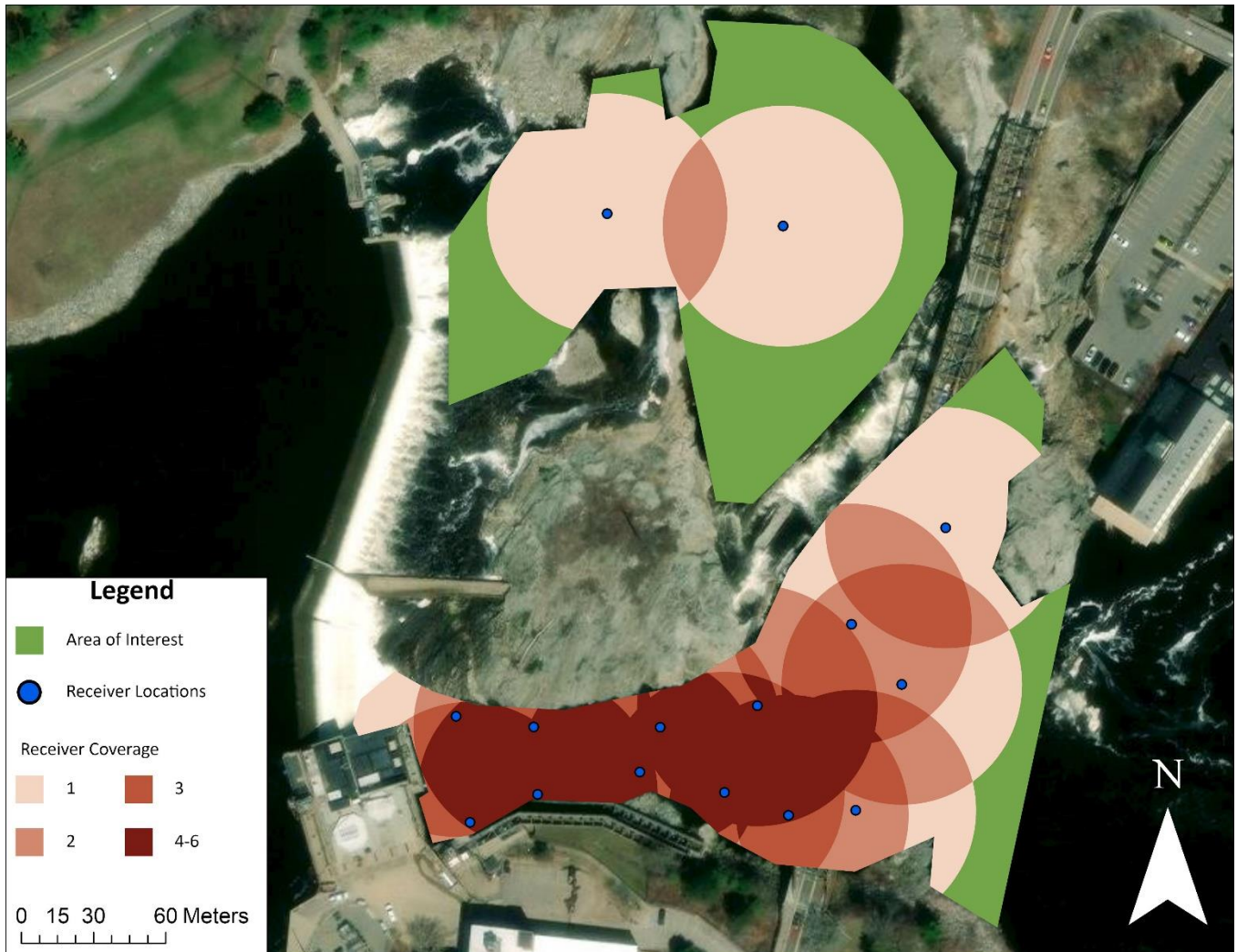
Figure 1. Example receiver configuration below the Brunswick Hydroelectric Project for use in the Diadromous Fish Behavior, Movement, and Project Interaction Study. Green is the assumed area of interest, and potential receiver locations are shown as blue circles. Receivers in this figure have an assumed range of 50 m, represented by the larger circles extending beyond receiver locations. The color of the larger circles represents the number of overlapping receivers covering a particular area, with dark colors indicating more receiver coverage. The literature suggests that simultaneous coverage of at least four receivers is needed to obtain accurate 3D locations for tagged fish. 7 The number of receivers indicated does not necessarily represent the maximum number of receivers needed for the study.
