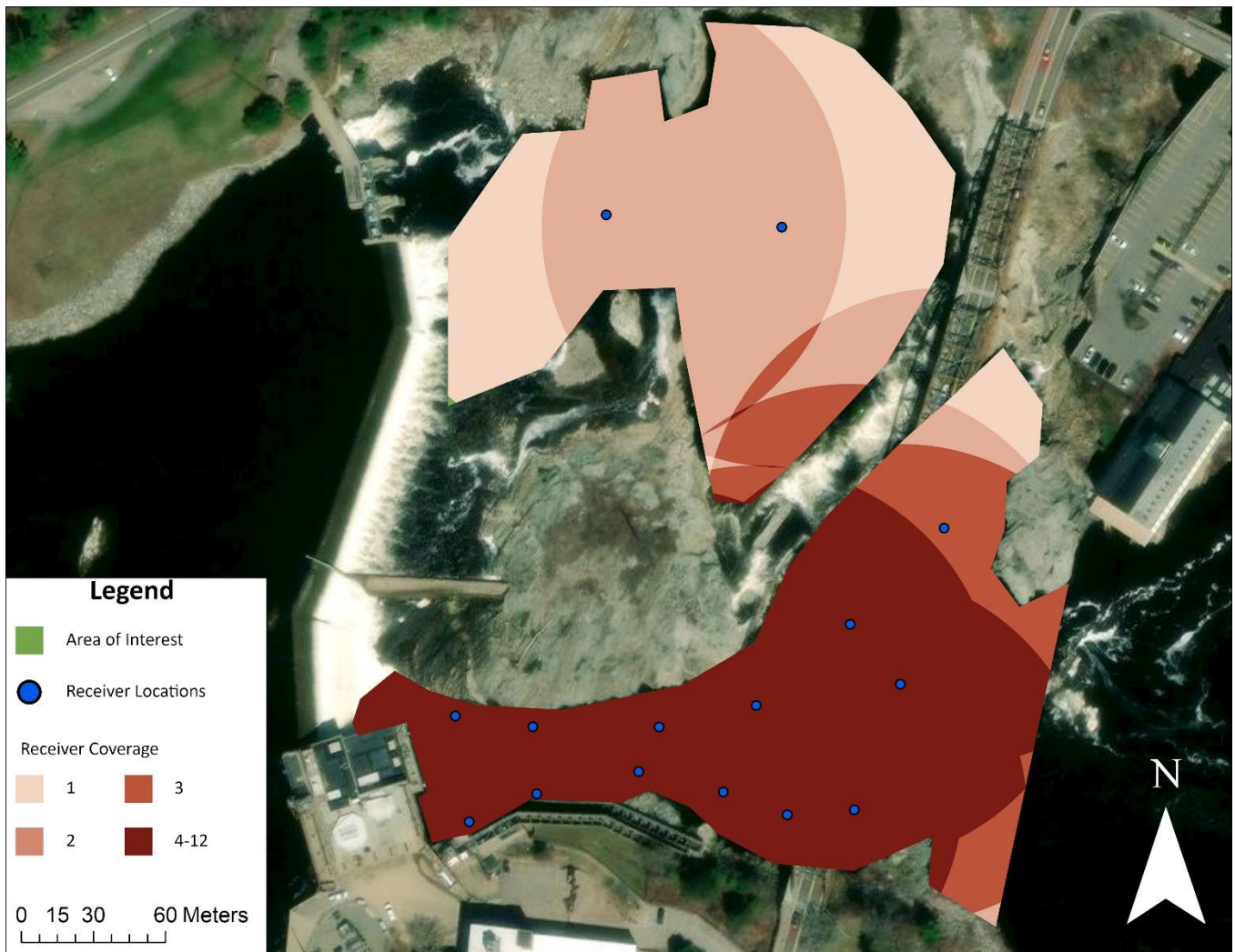
Figure 2. Example receiver configuration below the Brunswick Hydroelectric Project for use in the Diadromous Fish Behavior, Movement, and Project Interaction Study. Green is the assumed area of interest, and potential receiver locations are shown as blue circles. Receivers in this figure have an assumed range of 100 m, represented by the larger circles extending beyond receiver locations. The color of the larger circles represents the number of overlapping receivers covering a particular area, with dark colors indicating more receiver coverage. The literature suggests that simultaneous coverage of at least four receivers is needed to obtain accurate 3D locations for tagged fish. 8 The number of receivers indicated does not necessarily represent the maximum number of receivers needed for the study.
