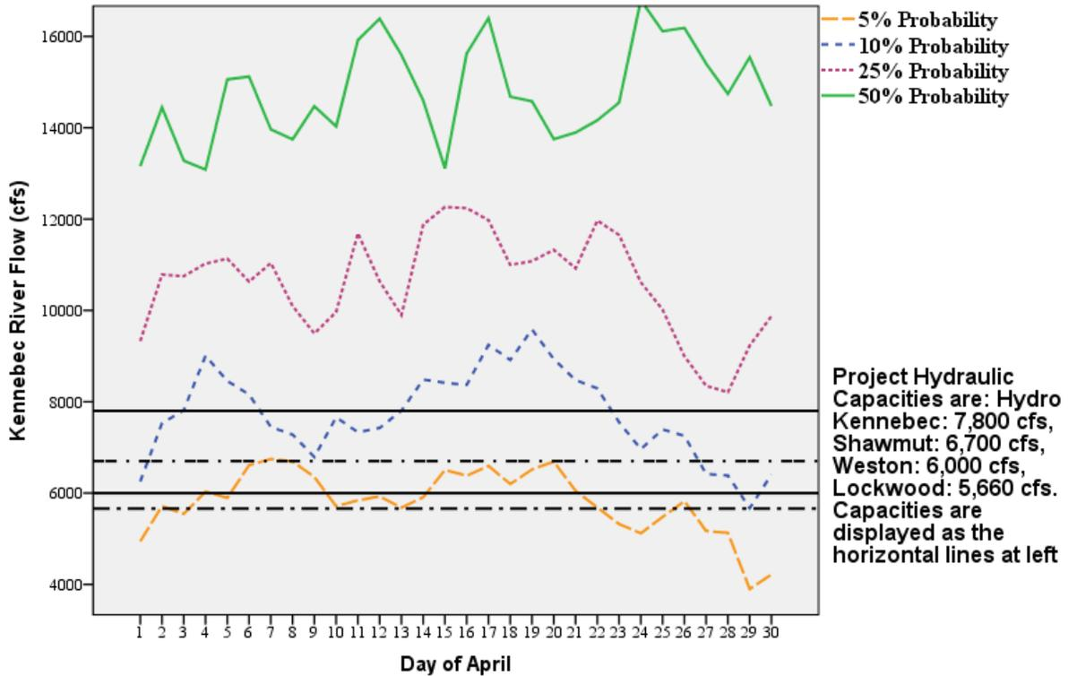
**Figure 7.1.1. Relationship between Kennebec River mean daily flow in April and the hydraulic flow capacity of the Hydro Kennebec, Shawmut, Weston, and Lockwood projects. Flow curves represent the 5, 10, 25, and 50<sup>th</sup> mean daily flow percentiles. Flow volume is based on all days of record for the USGS gage at North Sidney, ME with flows from the Sebasticook River at Pittsfield, ME subtracted. No flow adjustment has been made for changes in watershed area.**
