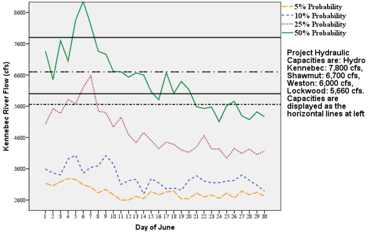
**Figure 7.1.3. Relationship between Kennebec River mean daily flow in April and the hydraulic flow capacity of the Hydro Kennebec, Shawmut, Weston, and Lockwood projects. Flow curves represent the 5, 10, 25, and 50<sup>th</sup> mean daily flow percentiles. Flow volume is based on all days of record for the USGS gage at North Sidney, ME with flows from the Sebasticook River at Pittsfield, ME subtracted. No flow adjustment has been made for changes in watershed area.**
