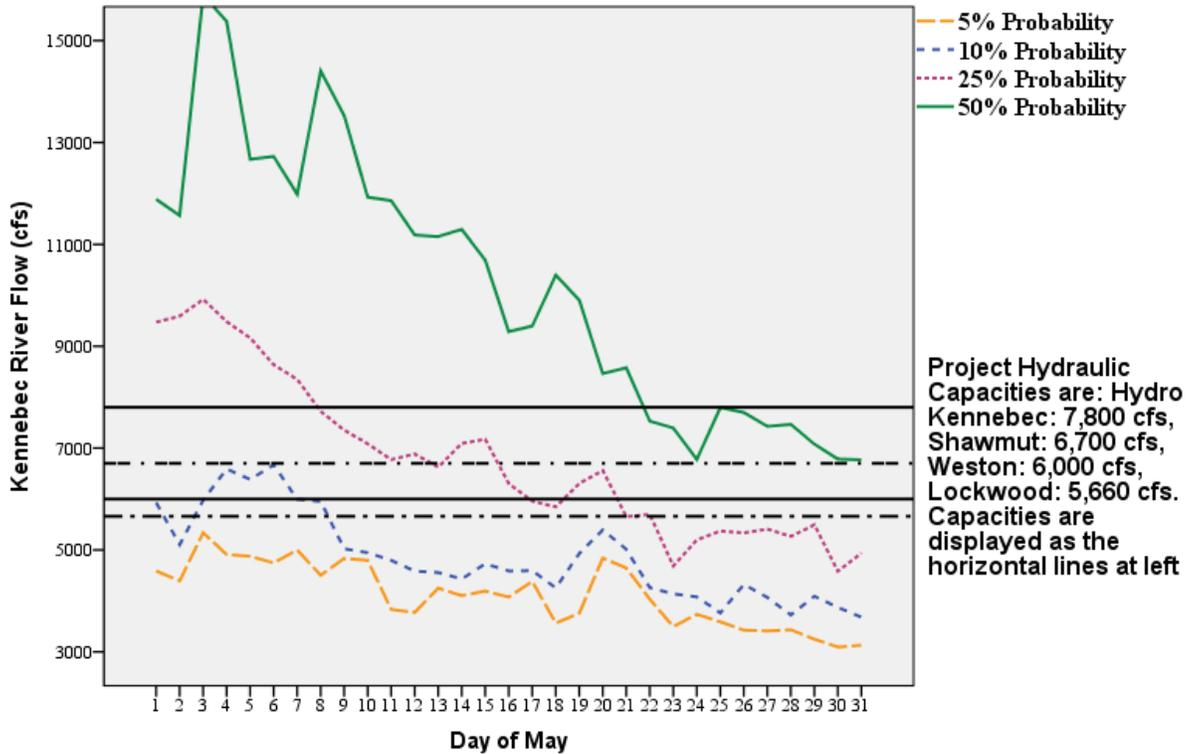
**Figure 7.1.2. Relationship between Kennebec River mean daily flow in April and the hydraulic flow capacity of the Hydro Kennebec, Shawmut, Weston, and Lockwood projects. Flow curves represent the 5, 10, 25, and 50<sup>th</sup> mean daily flow percentiles. Flow volume is based on all days of record for the USGS gage at North Sidney, ME with flows from the Sebasticook River at Pittsfield, ME subtracted. No flow adjustment has been made for changes in watershed area.**
