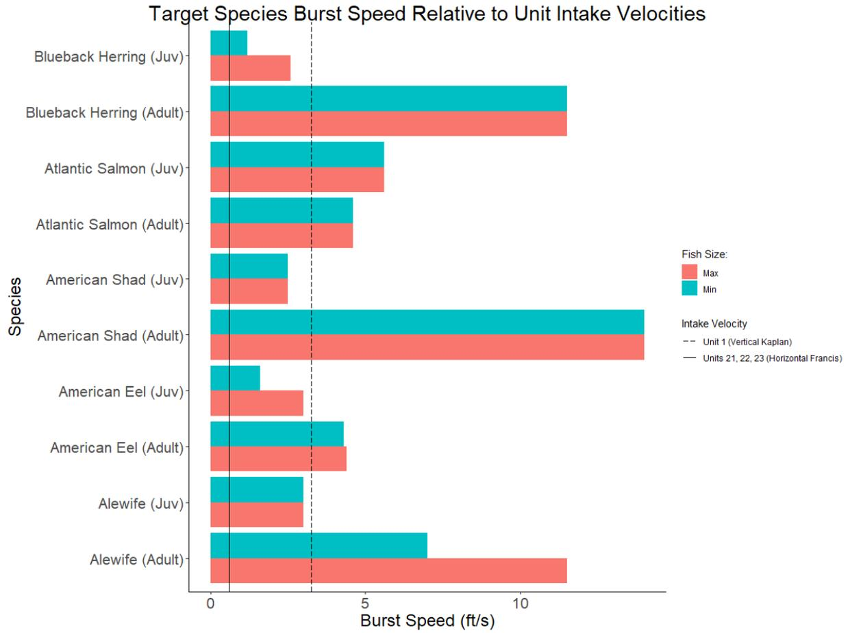
**Figure 4-3: Burst Swim Speed of Target Fish Species Compared to Approach Velocities Calculated for Project Intakes**
