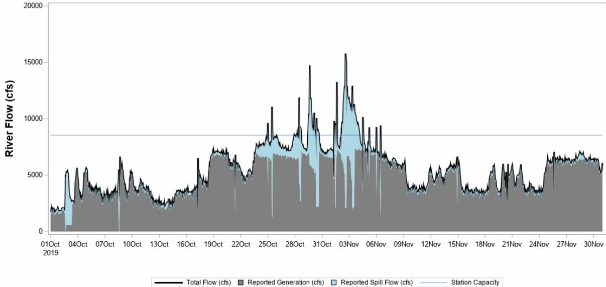
**Figure 5-2: Total, Powerhouse, and Spill Flow (cfs) Relative to Station Capacity at Pejepscot for the Period October 1 to November 30, 2019.**
